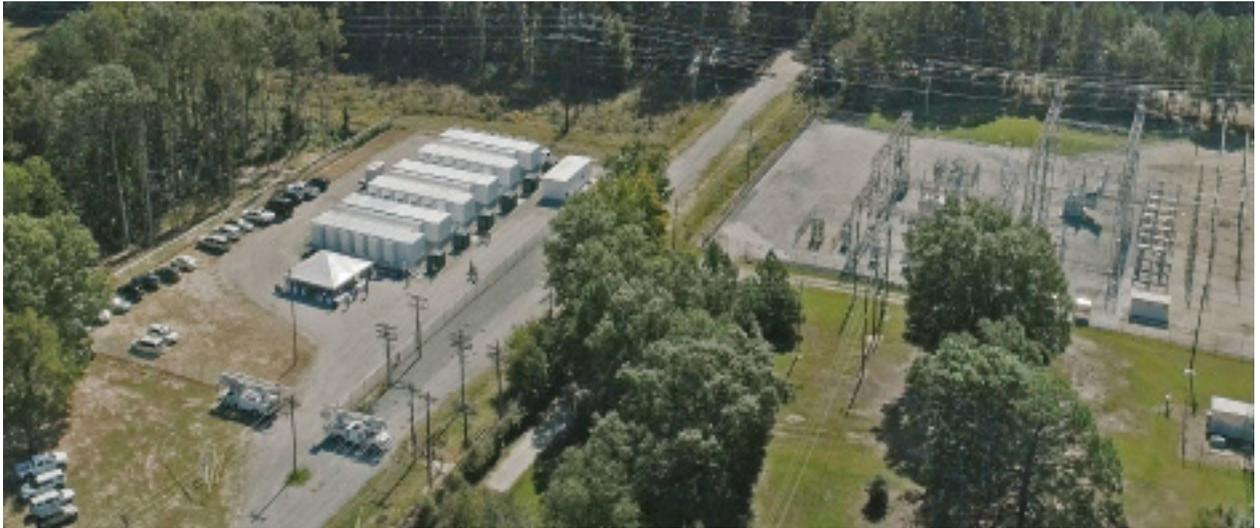
PowerBlock® generation concept, comprised of a standard container with between one and five standard engine generator sets, each powered by a Volvo 625kW Tier 4 Final engine and operating in parallel. Each PowerBlock flexibly adapts to the power needs of grocery stores, gas stations, community centers, hotels, and other C&I businesses with power ranges from 600kW to 3125kW.
