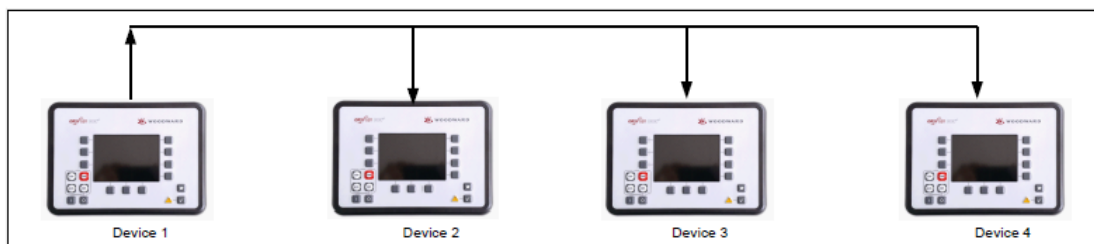
Fig. 269: Device 1 sends data to device 2, 3 and 4
