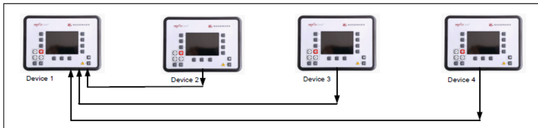
Fig. 270: Device 1 receives data from device 2, 3 and 4
