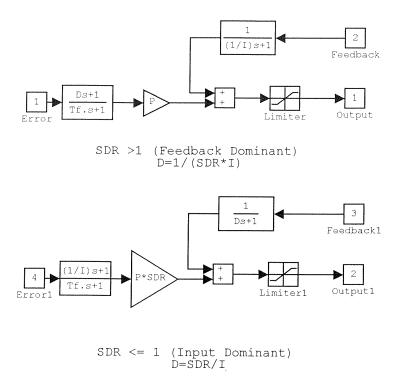
If SDR > = 100 then D and Tf are eliminated. For SDR < = .01 D and Tf are set to the same value and cancel each other out when the control is in use.
